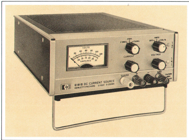
Fig. 3. New CCB Series, Models 6177B, 6181B and 6186B Current Sources, have their positive output terminals enclosed by a guard which eliminates most of the leakage currents shown in Fig. 2. They can supply currents as low as 1 \mu\text{A} , regulated within 25 ppm of setting \pm 5 ppm of range for a load voltage change from zero to maximum. They also have continuously adjustable voltage limits.
